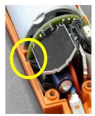
On the side edge of the motor electronics are two small cut-outs for laying the black cables for the Hall sensors (left).
