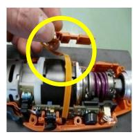
If the electronic strip and LEDs need to be replaced, first remove the defective electronic strip from the holder. To do this, carefully bend back the plastic hook and remove the display unit (left). Then insert the new display unit into the holder. The electronic strip is bent (centre) in order to insert it correctly into the tool. When fitting, make sure the bend is not too sharp as this could break the contacts (right)
