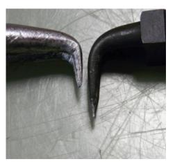
Before you can remove the circlip from the aluminium flange, you must release the spring with the adjusting ring up to its limit position. This will create enough space for you to reach the circlip with a pair of circlip pliers. However, a pair of standard circlip pliers must be ground down (picture on right).
