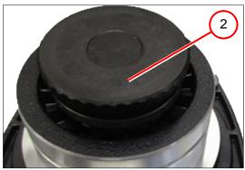
2. Remove the clamping unit (2).
