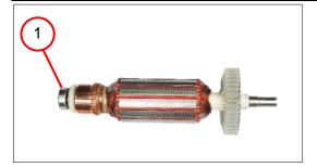
1. Press on the deep groove ball bearing (1).
