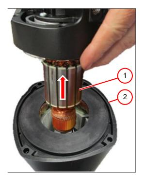
3. Remove the armature (1) from the motor housing (2).
