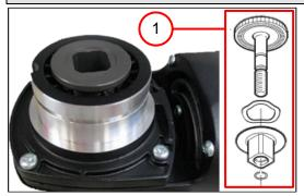
1. Positioning the clamping unit (1).
