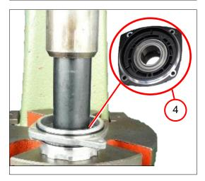
5. Press in the grooved ball bearing (4).
