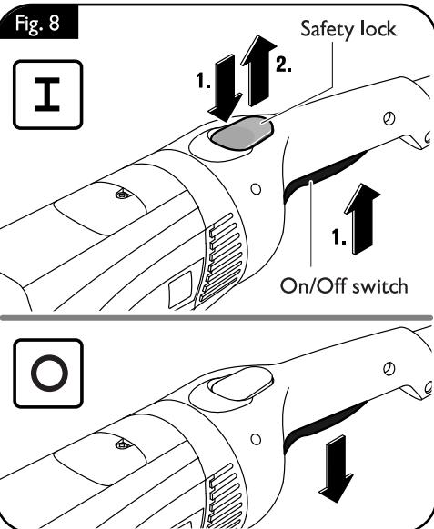
**Switching On with lock-on function:**
