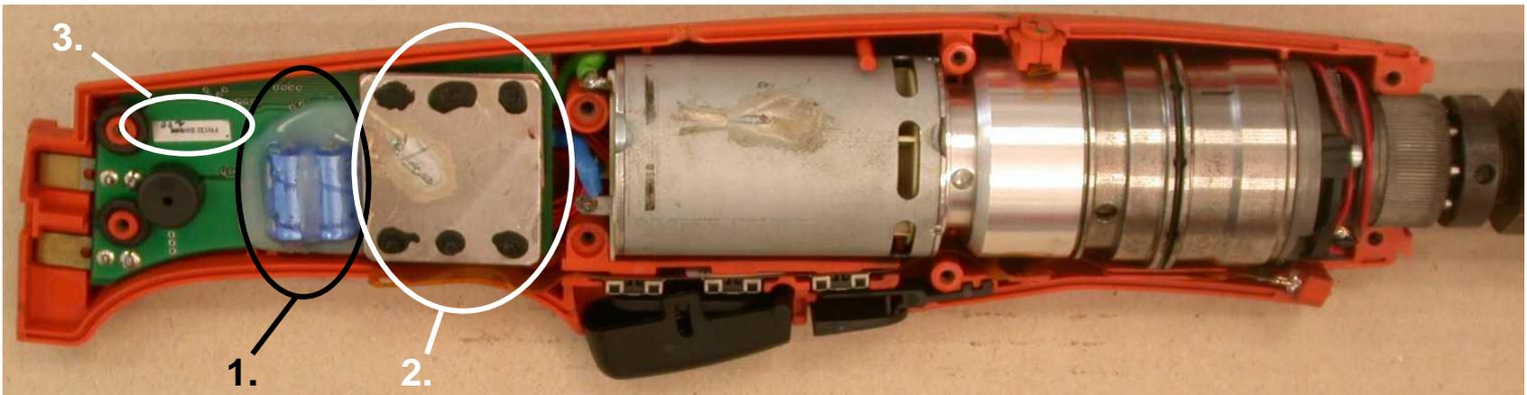
1. Glue capacitor C2 next to dissipator with hot-melt adhesive
