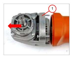
6. Remove the gearbox housing (1).
