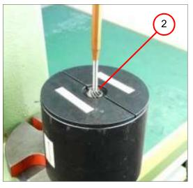
2. Remove the bevel pinion (2).
