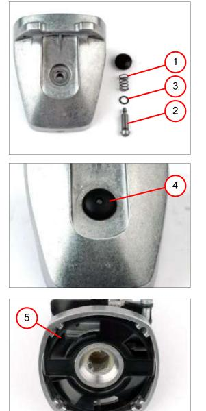
Insert the spiral spring (1) and the bolt (2) with sealing ring (3).
