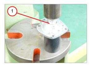
5. Press out the deep grooved ball bearing (1).
