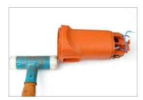
6. Remove the stator (1).
