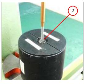
2. Remove the bevel pinion (2).
