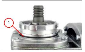
1. Remove the sealing ring (1).
