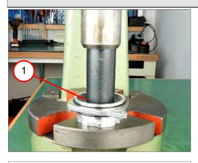
1. Press in the deep grooved ball bearing (1).
