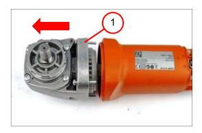
6. Remove the gearbox housing (1).
