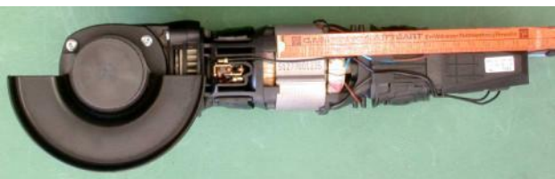
WSB 10-115 T: Field magnet in field magnet unit approx. 33mm long
