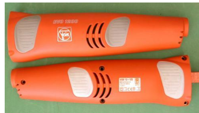
WSB 14-125 T: Motor housing approx. 265mm long
