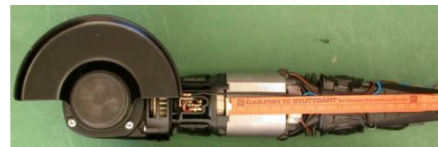
WSB 14-125 T: Field magnet in field magnet unit approx. 52mm long
