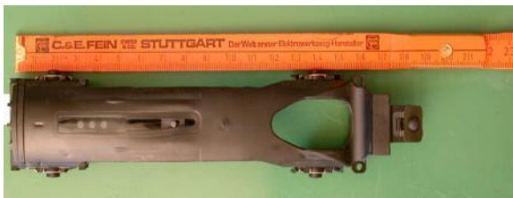
WSB 8-115: Switching module (60) approx. 190 mm long
