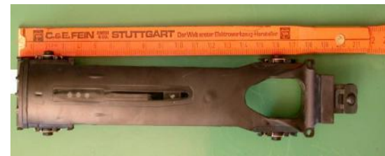
WSB 13-125: Switching module (60) approx. 210 mm long
