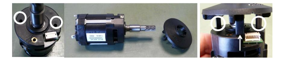
Warning – the bearing support can only be fitted in one position – see circles!!!!!!!! The third support must always be on the white terminal strip.
