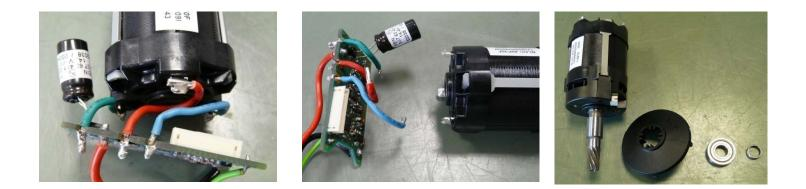
Unsolder electronics from motor – warning: note how the cables are laid!!!!! Remove grease wiper ring and ball bearing Remove bearing support
