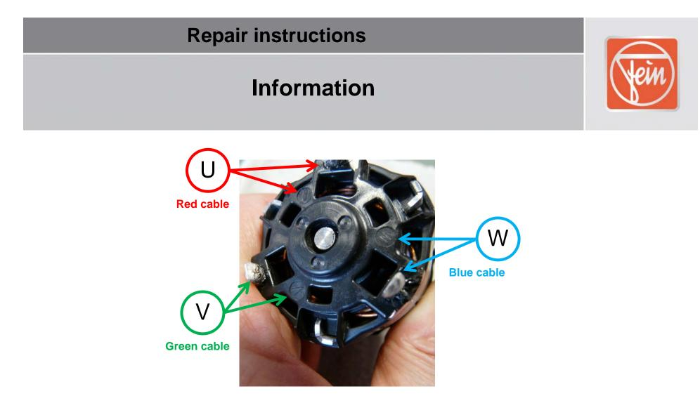
When soldering the cables to the motor, you must note the codes shown, otherwise the motor will not work.
