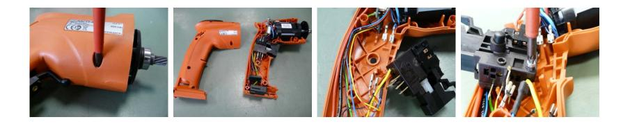
Loosen and remove screws on motor housing Remove upper section of housing Loosen switch contacts
