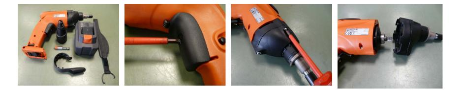
Remove battery, hook, wrist strap, depth stop sleeve and screwdriver bit Remove screw on pushbutton and pushbutton Loosen screws on gearbox housing and remove gearbox housing
