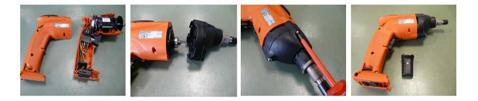
Position and screw down upper section of housing Place gear box head on tool and screw down Secure pushbutton on switch
