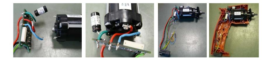
Solder electronics to motor Attach cable harness Insert wired motor and electronics into bottom section of housing
