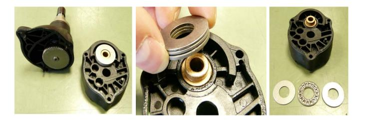
Remove intermediate bearing plate from gearbox housing Remove and replace needle cage and discs if necessary
