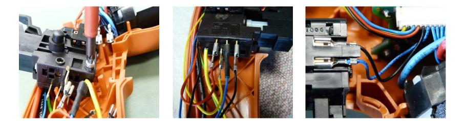
Secure yellow cable on switch's screw contact Connect plug contacts to switch -Note order of colours – otherwise the tool will not work
