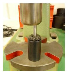
Remove clutch ring Press out second clutch ring
