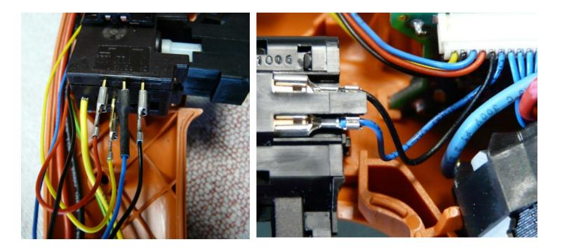
When changing switches, note the coloured connections, as otherwise the tool will not work or only have limited functionality
