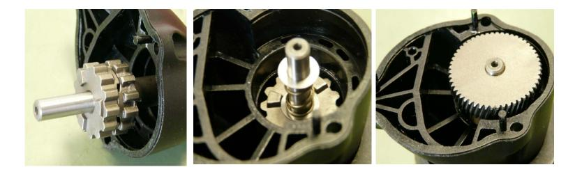
Insert shaft and clutch rings into gearbox housing Slide disc, spring and second disc onto shaft Slide gear-wheel onto shaft
