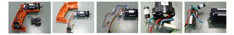
Remove switch Remove motor, electronics and connecting cable from motor housing Unsolder electronics from motor – warning: note how the cables are laid!!!!!
