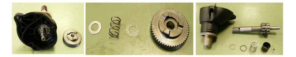
Remove gear-wheel, pressure spring and discs from shaft Disassemble tool mounting and remove shaft from gearbox housing
