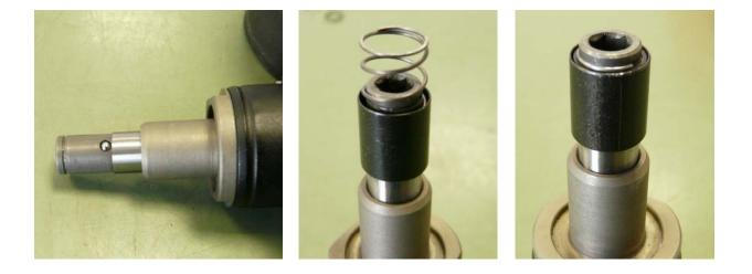
Place ball for fixing screwdriver bit into hole Slide sleeve and spring onto shaft (do not lose ball) Place spacer ring on spring and push everything downwards together Fit circlip – warning: this requires some patience because of the spring tension!!!
