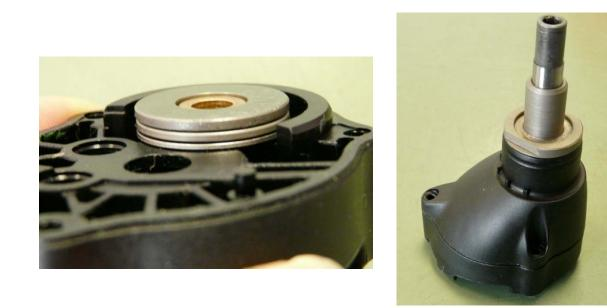
Place disc, axial bearing and second disc on plain bearing bush in intermediate bearing. Assemble shaft, intermediate bearing and gearbox housing
