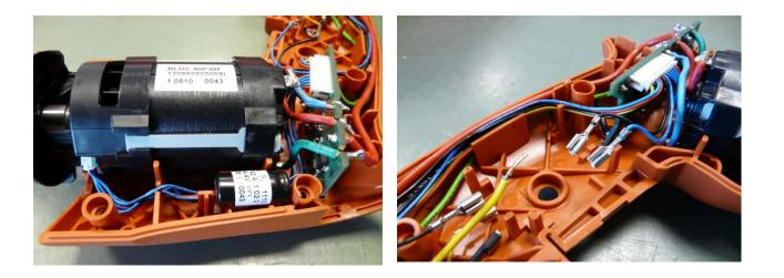
When inserting the motor and electronics, note how the cables are laid, cables must be laid underneath the suppression capacitor and must not be jammed.
