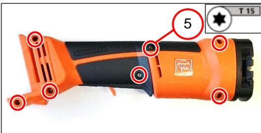
4. Screw in the seven screws (5) [1.5 Nm].
