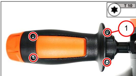
7. Screw in the four screws (1) [0.8 Nm].
