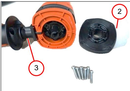
2. Remove the intermediate gear box (2).
