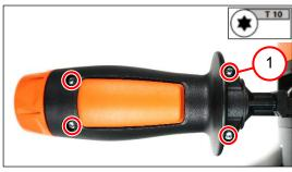
7. Screw in the four screws (1) [0.8 Nm].
