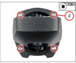
2. Screw in the four screws (2) [2.0 Nm].
