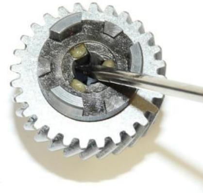
1. Monter le circlips.
