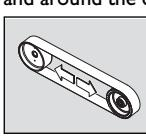
Tilt lever (5) down to tension the grinding belt.
