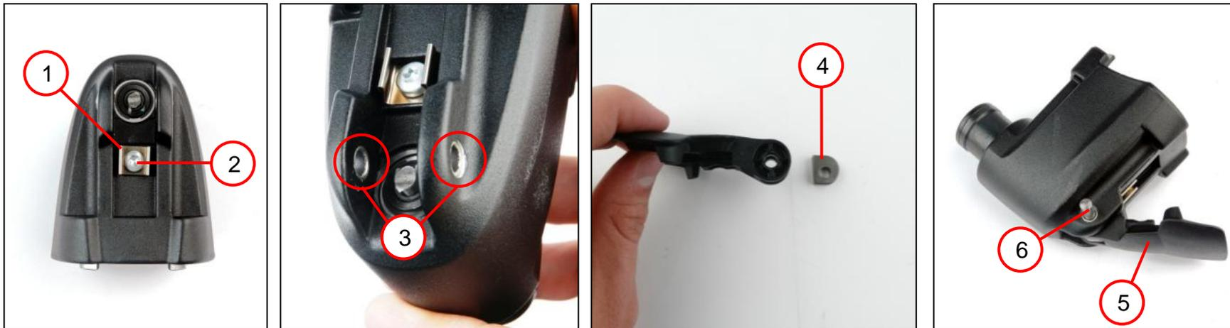
1. Secure locking spring (1) with fillister head screw (2) [2.0 ±0.1Nm].
