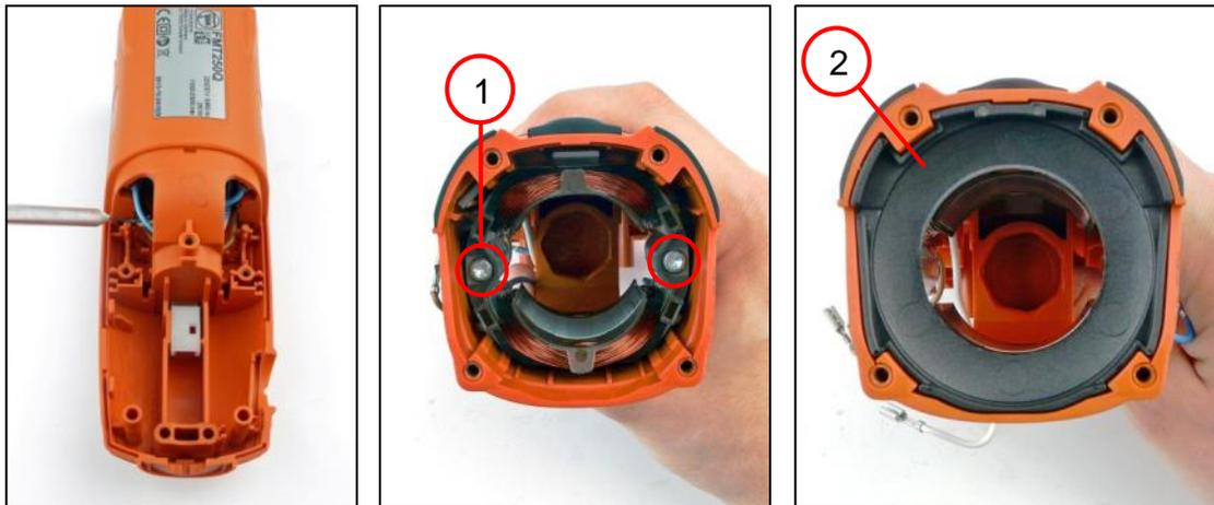
1. Using hook, pull cables out of stator.
