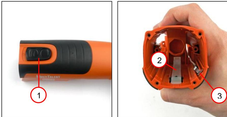
1. Clip slide switch (1) into motor housing.
