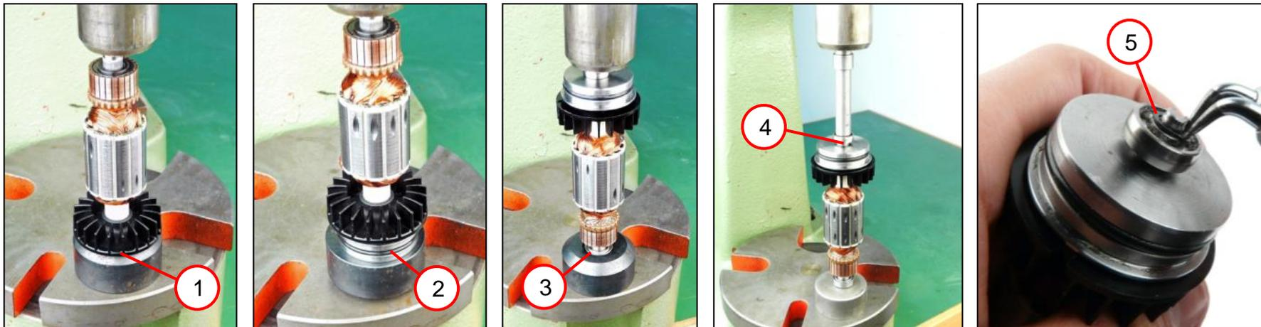
1. Press on grooved ball bearing (1).
