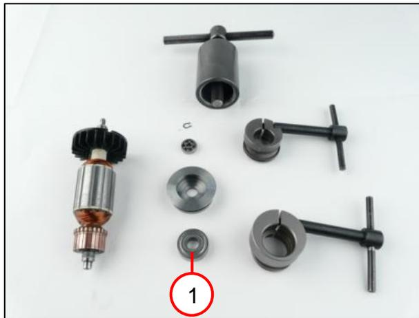
1. Pull ball bearing (1) off armature.
