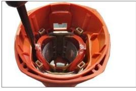
5. Press down the contact spring with the assembly aid.
