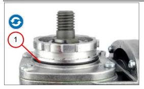
1. Remove the sealing ring (1).
