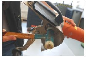
5. Remove the grinding arm (5).
