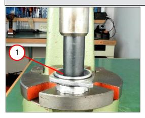
1. Press in the grooved ball bearing (1).
