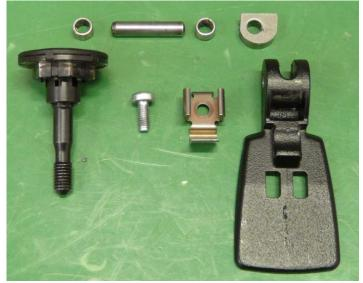
Because of the specifications for the press-in force of the drive shaft, which cannot be guaranteed after repairs, the gear box head is only replaced as a complete assembly and offered as a complete spare part.
