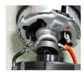
Attach switch spring to electronics. Solder electronics to motor.
