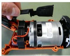
Remove screws from motor housing. Cut through centre of type plate. Remove upper section of housing. Remove control rod.
