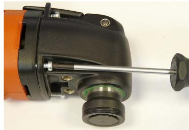
Fill gear box head with grease (8 g). (Lubricant ID: 32160003014)
