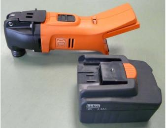
Press releasing button and remove battery.
