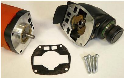
Remove screws from gear box head. Remove gear box head. Remove seal.
