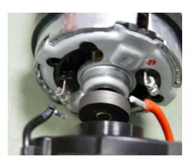
Remove motor with electronics and intermediate bearing from lower section of housing. Unsolder electronics.
