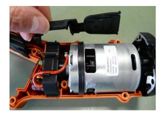
Insert motor with electronics and intermediate bearing into lower section of housing. NOTE: Motor must sit in centring fixture in lower housing section.
