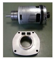
Carefully press motor out of intermediate bearing.
