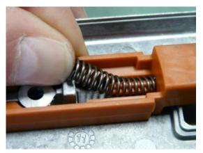
1. Insert pushbutton with attached pressure spring into housing
