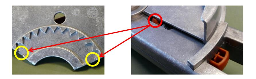
To dismantle the spark hood, when the pushbutton is pressed into the middle position, the pushbutton pin is level with the openings on the bottom of the spark hood. The spark hood can therefore be dismantled on both sides (red circle and arrow – left or right opening).
