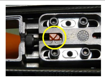
The correct belt tension is set using the clamping screw on the clamping sleeve assembly. It is achieved when the two marks are directly opposite one another. (Yellow circle)
