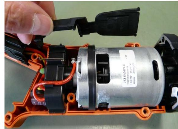
Insert motor with electronics and intermediate bearing into lower section of housing.
