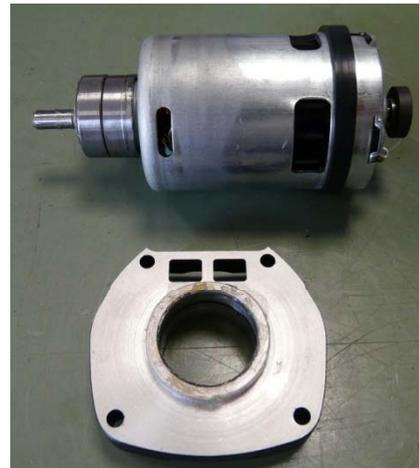
Carefully press motor out of intermediate bearing.
