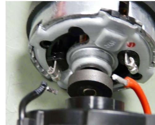
Remove motor with electronics and intermediate bearing from lower section of housing.
