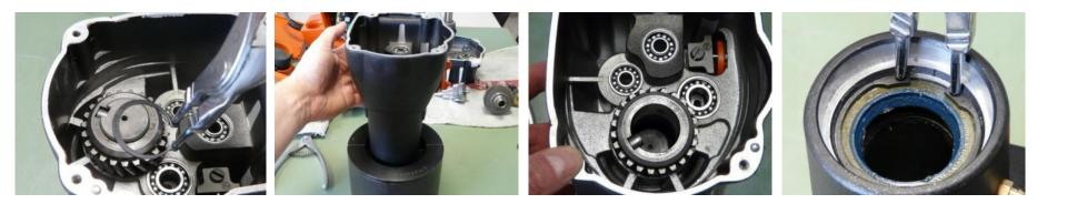
Remove circlip from drill shaft gear-wheel Press drill shaft out of gearbox housing using a press-out sleeve, remove gear-wheel with feather key
