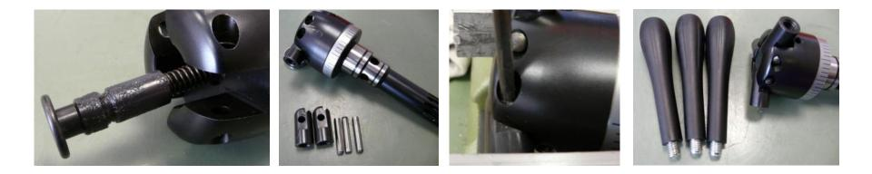
Insert selector shaft into shaft Insert switch bar and fix with dowel pin Screw handles into switch bolts
