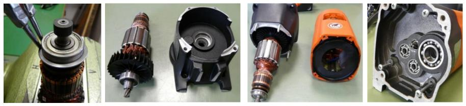
Press-fit ball bearing and magnet ring Attach spacer to bearing Attach armature to intermediate bearing and press in Insert assembled intermediate bearing in motor housing and secure with 4 screws Fill gearbox with grease (350 g – 3 21 320 07 18 9) Stick the Gearbox with Loctite 5188 Close the Gearbox with the 4 screws
