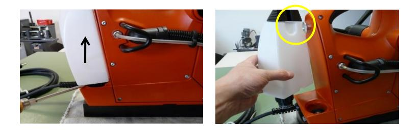
Lift coolant tank up with screwdriver and pull upwards by hand until tank is disengaged from lock at top end. (Yellow circle) The tank can then be removed from the tool.
