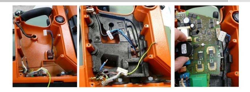
Place bottom part of foam in drill jig Insert electronics in foam
