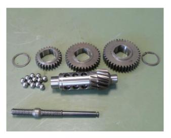
Dismantle large intermediate gear – the three gearwheels that switch the gears are slid up and are fixed or released by the balls depending on the gear selected Remove gear-wheels and balls Remove control rod
