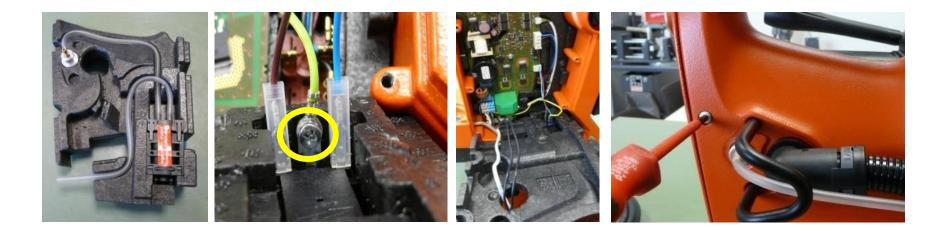
Insert coolant pump, hoses and distributor in foam cover Connect earthing conductor contact to coolant pump Insert motor cable through opening Attach foam cover and metal cover and screw down
