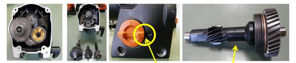
Remove grease from gearbox Remove intermediate gear from gearbox housing Warning – it is best to remove the large intermediate gear when the gear converter is in first gear Warning – the intermediate gear with slipping clutch is only available as a complete spare part, because the slipping clutch is pre-set
