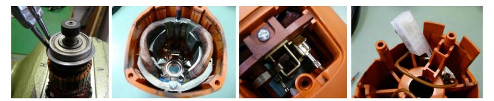
Remove spacer (if necessary) from ball bearing with circlip pliers Carefully press out magnet ring (risk of breakage) Remove bearing and replace if necessary Remove 2 screws from field coil Remove plug connection (brown cable) from carbon holder Remove contact plug (white) from holder and slowly pull out of motor housing with field coil (to do this, all cables must be routed between the ribs of the housing)
