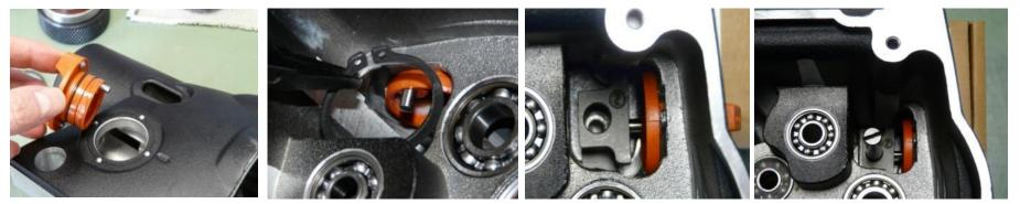
Insert switching handle and secure with circlip Place shifting claw in housing and move switching handle pin into guide
