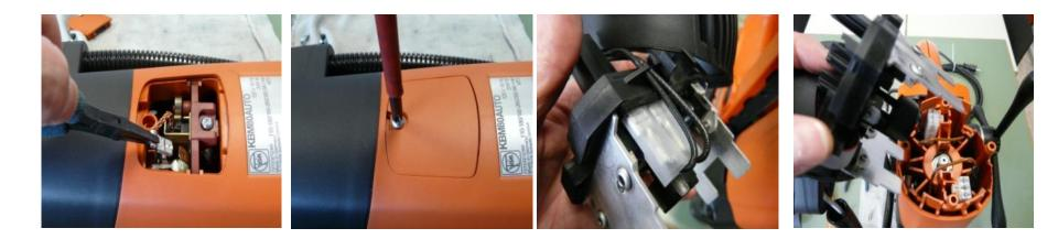
Insert and connect carbon brushes Fit both carbon brush covers Connect motor electronics and place in motor housing
