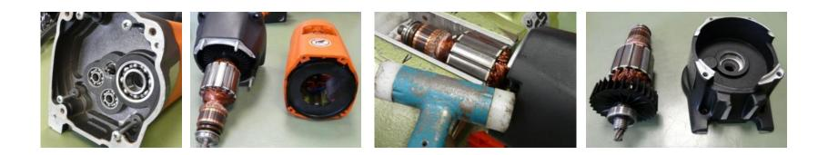
Loosen 4 screws on intermediate bearing Remove intermediate bearing with armature from motor housing Clamp armature in vice with aluminium jaws Disconnect intermediate bearing from armature by striking with hammer
