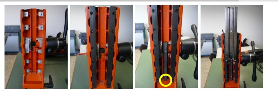
Put in the gliding bars to the drill jig and feed the screws (not tighten) Lay in the gear rod to the gear teeth of the gear box (locking pin down – yellow circle) Move down the guide from the upper side
