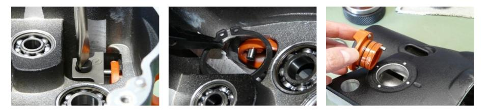
Loosen screw for securing shifting claw and remove shifting claw – best done in first gear switch position Remove circlip for securing switching handle and remove switching handle. Replace if necessary
