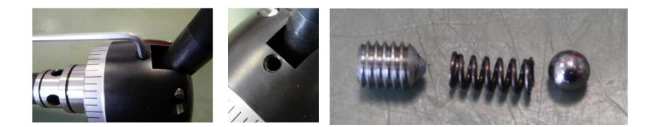
Remove set screw Remove spring and ball
