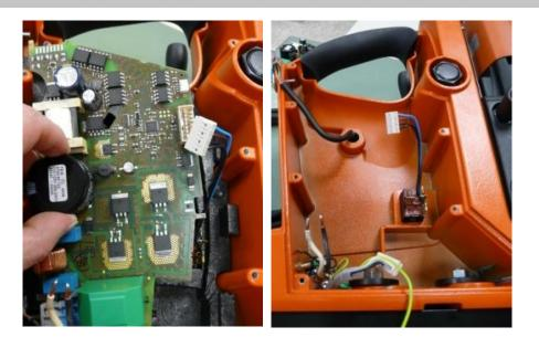
After all the connections from the circuit board to the switches and other components have been disconnected, the circuit board can now be removed from the foam and the drill jig.
