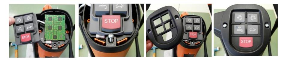
Insert console electronics into holder and attach rubber safety shutdown mat Secure plastic housing with 2 screws Attach and screw down cover – warning, check that pushbutton is secure, it must not jam !!!
