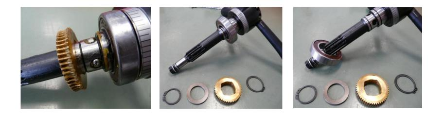
Remove worm wheel from drive shaft Remove balls Remove circlip Prise ball bearing out of bearing seat with screwdriver
