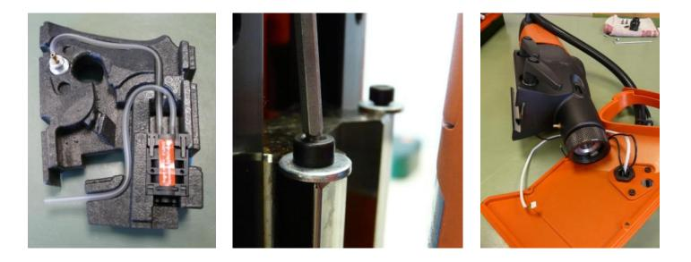
Remove electronics cover with coolant pump and hoses Loosen and remove screws for fall protection on dove-tail guide Remove cover of drill jig and drill motor from drill jig
