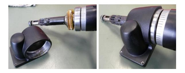
Slide housing over bearing as far as stop by gently striking with the hammer
