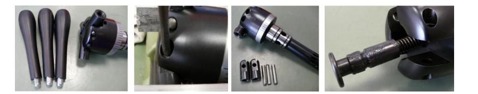
Unscrew handles Drive out dowel pins with punch Remove switch bar Remove control rod from drive shaft
