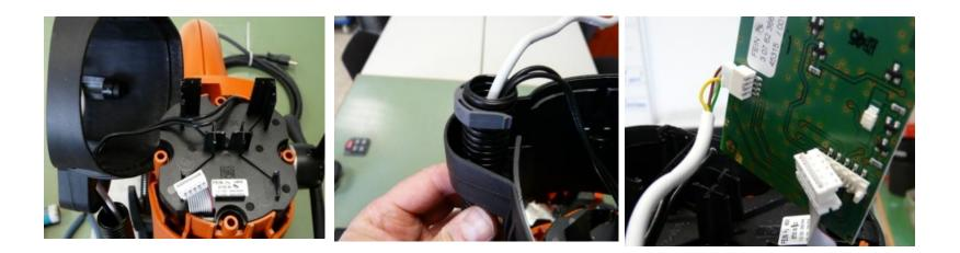
Attach plastic housing Insert protective hose with connection cables and lock Connect white speed cable and ribbon cable to console electronics
