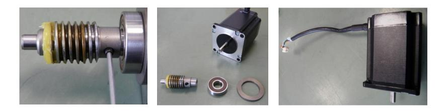
Loosen set screw Remove worm with ball bearing and spacer from motor shaft Feed motor is only available as a spare part in complete form (see photo on right)
