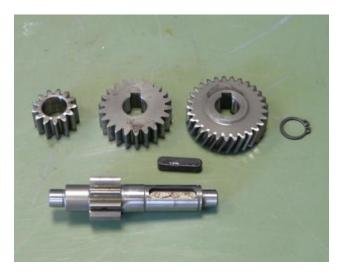
Dismantle small intermediate gear – the two large gear-wheels are slid up and are guided through the feather key, the small gear-wheel is press-fitted. The press fitting is damaged when the small gear-wheel is disassembled. The gear-wheel and the shaft cannot be used again as a result. The specified torque can no longer be transferred.
