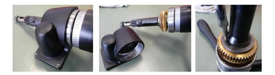
Remove housing from bearing by gently striking with plastic hammer Remove circlip
