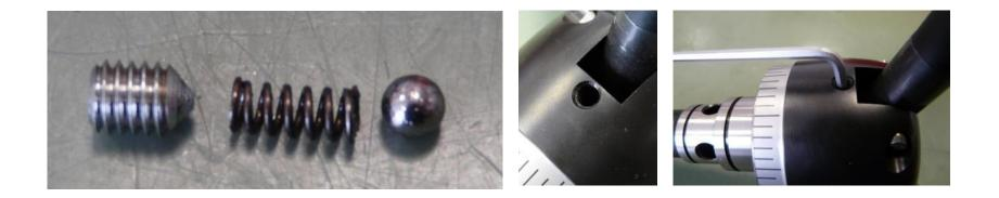
Insert ball, spring and set screw Fix set screw manually – must not compress solid, otherwise automatic function will not work
