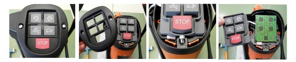
Remove 2 screws from cover cap Remove cover Loosen and remove screw for securing housing Remove safety shutdown mat
