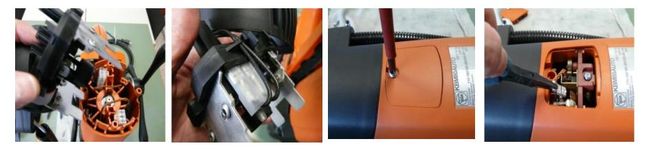
Remove motor electronics from motor housing Remove both plug contacts from motor electronics Loosen screw on carbon holder cover and remove carbon holder cover Pull plug contact out of carbon brush and remove carbon brush
