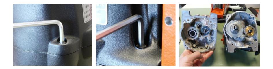
Loosen 4 screws on gearbox housing Remove gearbox housing (careful, it is bonded with Loctite 5188 surface seal) Remove and replace grease
