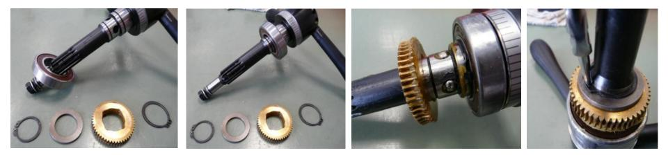
Slide ball bearing on to shaft and press-fit, secure with circlip Insert balls, slide on gear-wheel, spacer and secure with circlip
