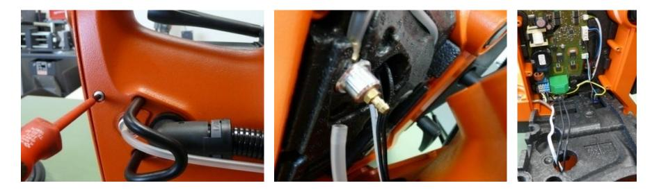
Remove screws from cover of drill jig. Pull out coolant hose. Fold metal cover and foam cover forwards and down.
