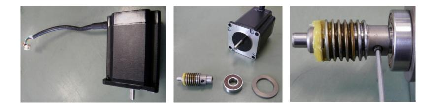
Complete feed motor with spacer, ball bearing and worm wheel The worm wheel is secured to the feed motor shaft with a set screw. The shaft has a milled groove on one side with which the set screw <u>must</u> come into contact.
