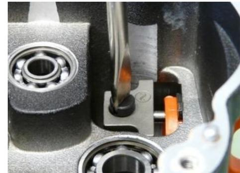
**Insert switching handle and secure with circlip
