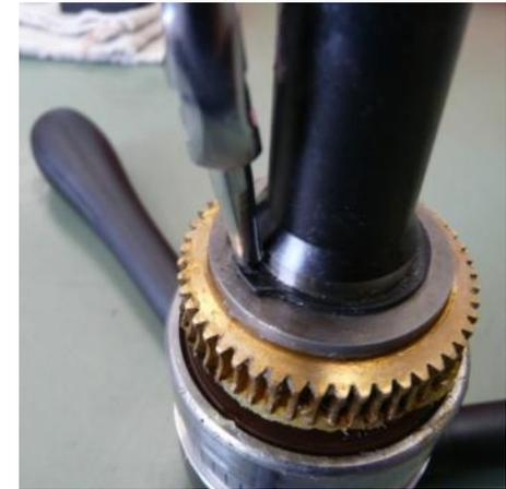
**Remove housing from bearing by gently striking with plastic hammer
