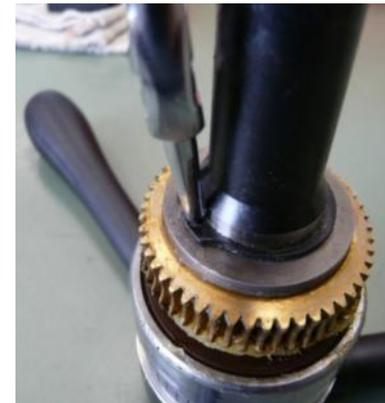
**Slide ball bearing on to shaft and press-fit, secure with circlip
