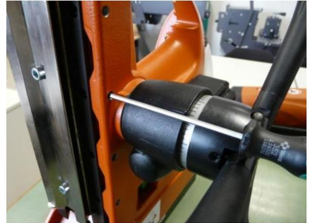
**Move up the gear rod with the gear teeth of the gear box until the screw holes match together**
