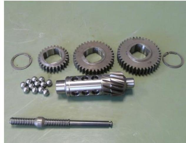
**Dismantle large intermediate gear – the three gear-wheels that switch the gears are slid up and are fixed or released by the balls depending on the gear selected
