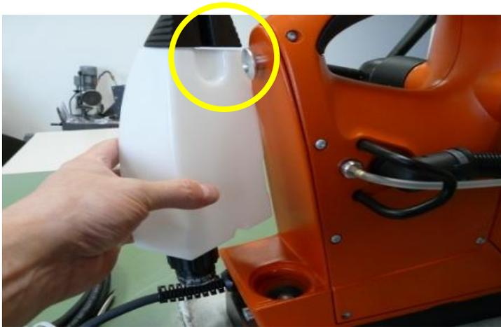
**Place coolant tank on top guide (yellow circle) and then press down**
