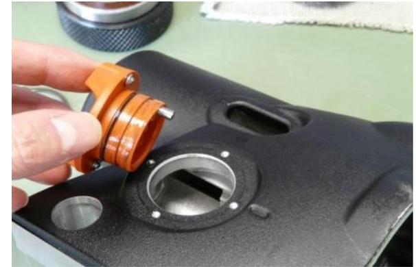
**Loosen screw for securing shifting claw and remove shifting claw
