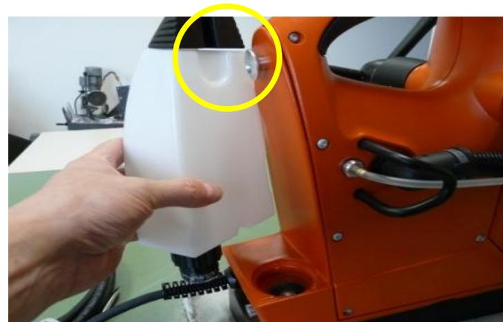
**Lift coolant tank up with screwdriver and pull upwards by hand until tank is disengaged from lock at top end. (Yellow circle)
