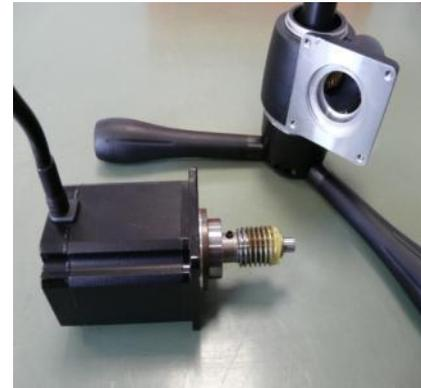
**Remove screws from motor fastening**
