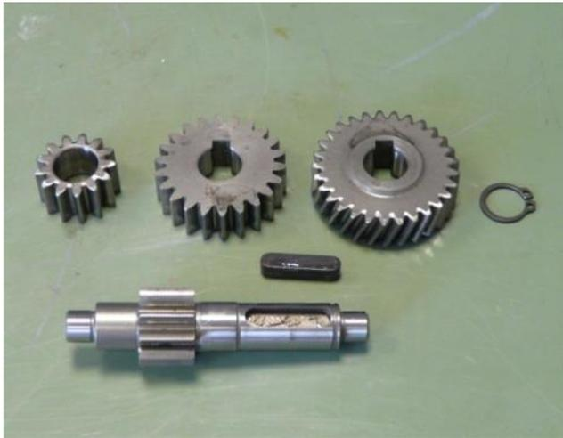
**Dismantle small intermediate gear – the two large gear-wheels are slid up and are guided through the feather key, the small gear-wheel is press-fitted. The press fitting is damaged when the small gear-wheel is disassembled. The gear-wheel and the shaft cannot be used again as a result. The specified torque can no longer be transferred.**
