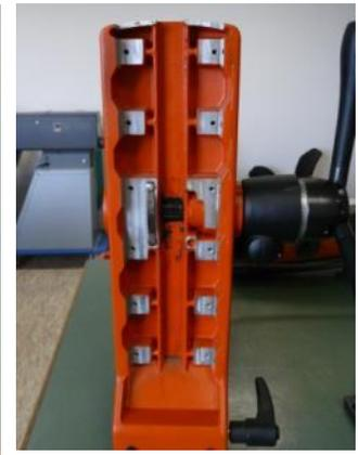
**Loosen the two screws on the guide and take it off.**
