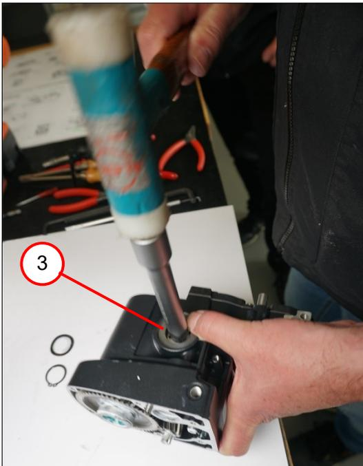
3. Remove the feed shaft (3).
