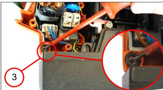
3. Remove the sealing ring (3).
