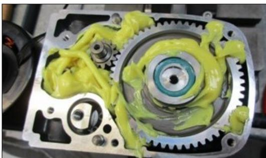
8. Fill the gearbox with grease.
