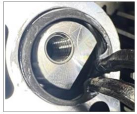
3. Position the circlip (3).
