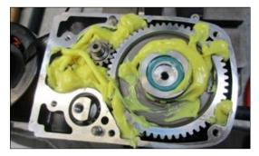
8. Fill the gearbox with grease.
