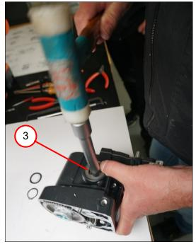
Remove the feed shaft (3).
