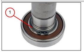
1. Remove the circlip (1).
