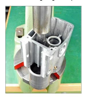
9. Press in the two deep groove ball bearings (1).
