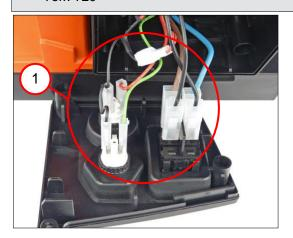
Connect all plug connections (1) as shown in the connection diagram.
