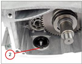
6. Position the circlip (2).
