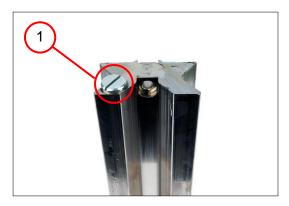
7. Screw in the flat-head screw (1) [1.2 Nm ±0.15 Nm].
