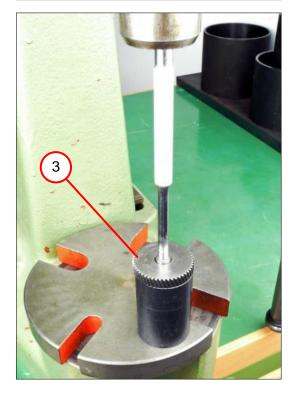
7. Press the gearwheel (3) off the shaft.
