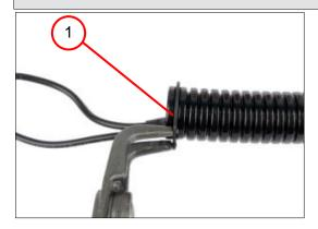
1. Remove the circlip (1).
