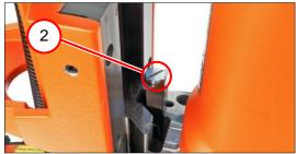
4. Screw in the flat-head screw (2) [1.2 Nm ±0.15 Nm].
