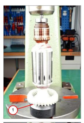
3. Press on the deep groove ball bearing (1).
