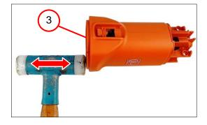
3. Remove the stator (3).
