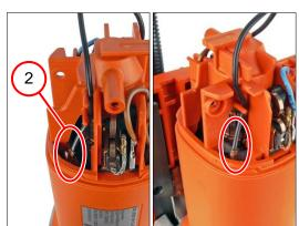
2. Connect the two strands (2) as shown in the connection diagram.
