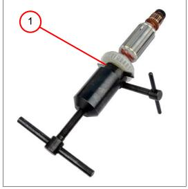
1. Remove the deep groove ball bearing (1).
