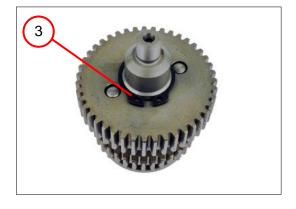
4. Remove the circlip (3).
