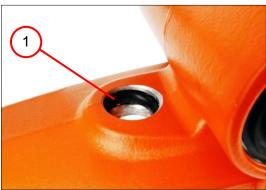
2. Remove the sealing ring (2).
