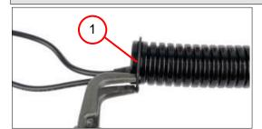
1. Position the circlip (1).
