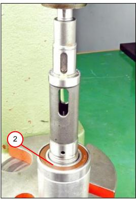
2. Press the deep groove ball bearing (2) off the shaft.
