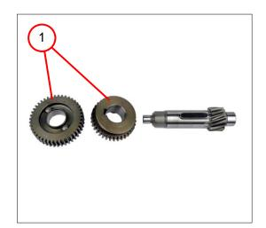
5. Remove the two gearwheels (1).
