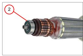
2. Remove the deep groove ball bearing (2).
