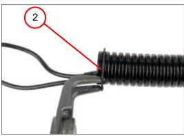
2. Position the circlip (2).
