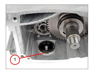
1. Remove the circlip (1).
