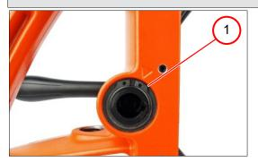
1. Remove the circlip (1).
