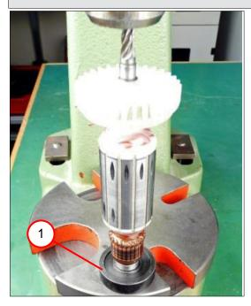
1. Press on the deep groove ball bearing (1).
