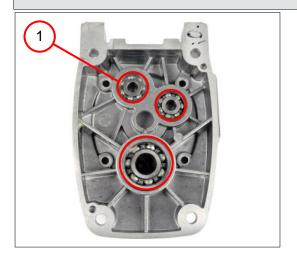
1. Press in the deep groove ball bearings (1).
