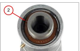
3. Position the circlip (2).
