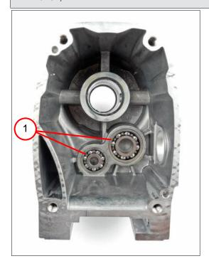
1. Remove the two deep groove ball bearings (1).
