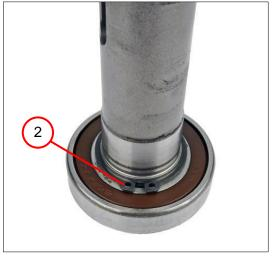
2. Position the circlip (2).
