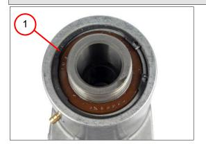
1. Remove the circlip (1).
