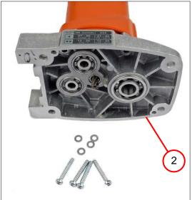
2. Remove the intermediate gear box (2).
