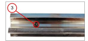
10. Screw in the screw (3) [3.0 Nm ±0.3 Nm].
