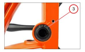
4. Position the circlip (3).
