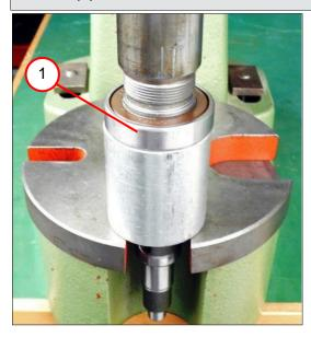
1. Press on the deep groove ball bearing (1).
