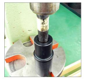
4. Press in the circlip (5).
