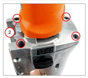
2. Screw in the four screws (2) [8.0 Nm ±0.3 Nm].
