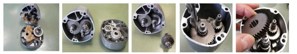
Disconnect gearbox housing and intermediate bearing. Remove grease. If the slipping clutch remains in the gearbox housing when the two housings are separated, take it out at this point. Remove circlip from gear-wheel. Take out gear-wheel.
