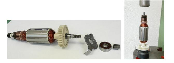
Slide plate on to armature shaft Press on ball bearing. Press on sealing ring. Press ball bearing onto collector side. Attach plastic bush along with magnet ring. Drive in gearbox housing.
