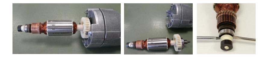
Drive armature out of intermediate bearing by tapping gently with a plastic hammer. Prise off plastic bush along with magnet ring. Pull out ball bearing.
