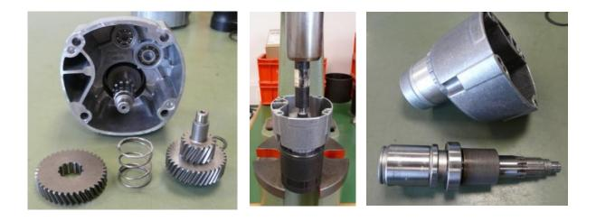
Remove pressure spring and intermediate gear. Press drill shaft out of gearbox housing.
