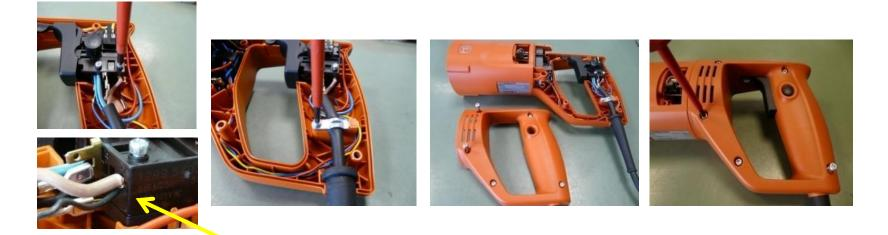
Fit mains cable with stranded wire for restart protection (thin black cable) Fit traction relief for mains cable Attach top handle half shell and screw down
