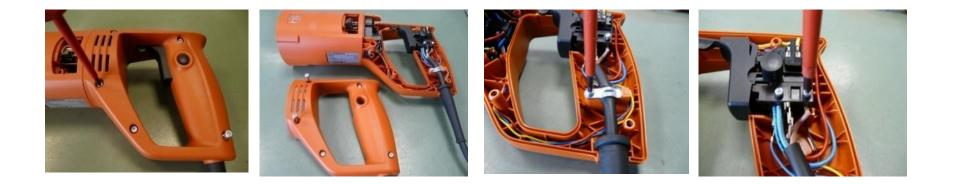
Loosen screws and take off handle half shell. Unscrew cable clamping bridge for cable. Loosen screw connection from cable on switch and take out cable.
