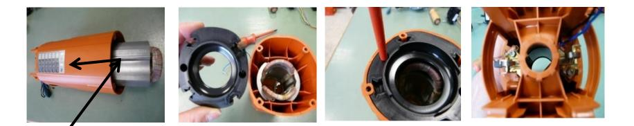
Insert field coil up to stop in motor housing -
