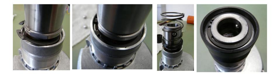
Fix drill shaft in gearbox housing with circlip Rotate drill shaft until the wrench flat provides good access for inserting the circlip Attach ring, insert balls, fit pressure spring Attach sleeve and press down Attach disc and insert circlip
