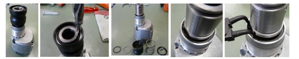
Place gearbox housing on intermediate bearing.
