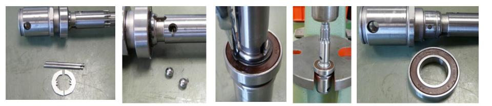
Pull both bolts out of drill shaft from the front. Remove the two balls. Remove circlip on ball bearing. Press ball bearing down and off drill shaft.
