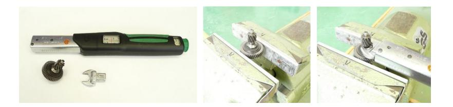
Clamp slipping clutch in vice with aluminium jaws.
