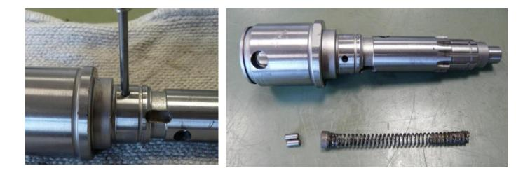
Use a punch to drive in fastening bolt. Remove spring.
