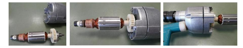
Insert armature in gearbox housing and drive in by tapping the housing gently.
