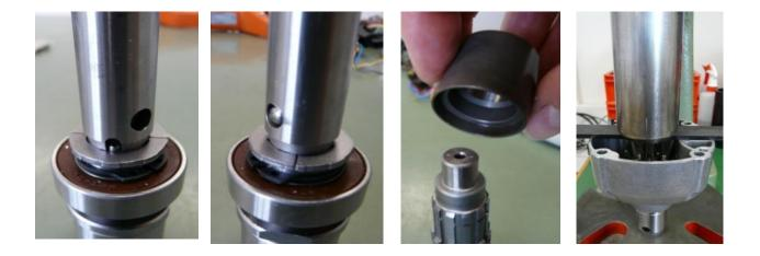
Insert circlips. Insert the two balls with a little grease. Fit sliding sleeve. Press drill shaft into outer bearing.
