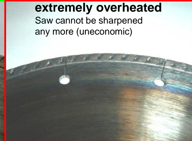
extremely overheated with contour deformation
