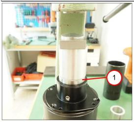
1. Press in the grooved ball bearings (1).
