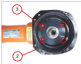
Position the housing (2) correctly.
