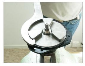
1. Secure the bearing housing (1) with the mounting device.
