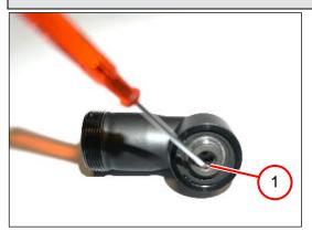
1. Position the circlip (1).
