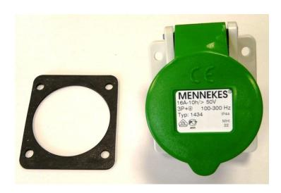
When replacing the socket, do not forget the rubber seal and ensure correct connection. L1 = black, L2 = grey, L3 = white, SL = yellow/green
