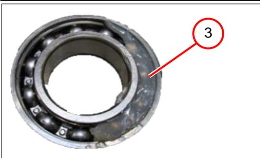
4. Grease the grooved ball bearing (3).
