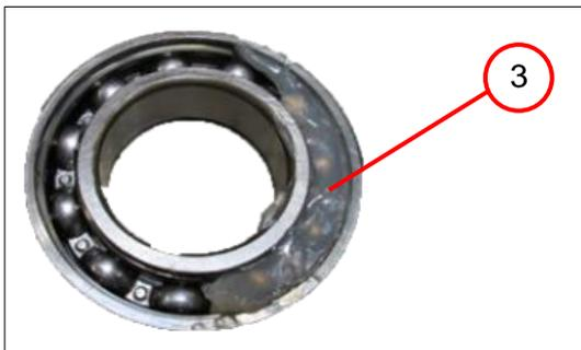
4. Grease the grooved ball bearing (3).
