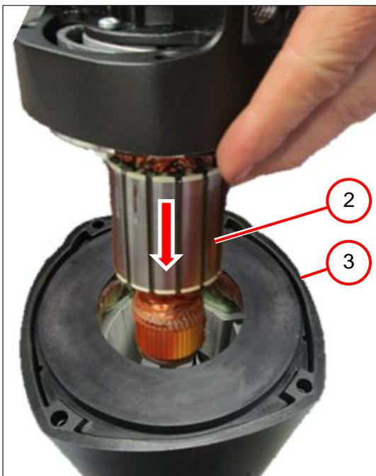
2. Position the armature (2) in the motor housing (3).
