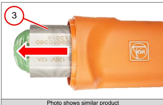
6. Remove the stator (3).
