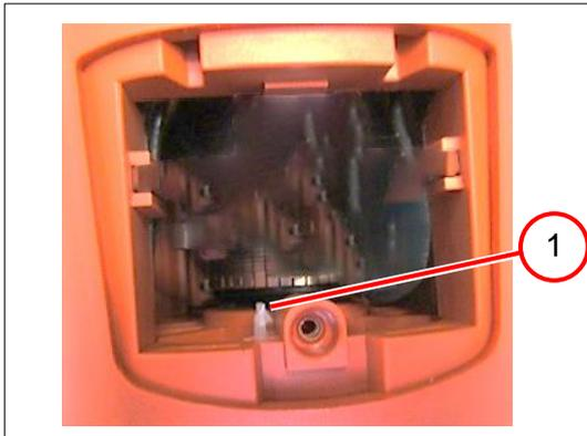
3. WSG 20/25-180/230: Loosen the locking mechanism (1).
