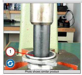
1. Press in the grooved ball bearing (1).
