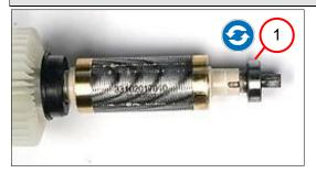
1. Press on the deep groove ball bearing (1).
