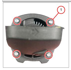
1. Screw in the four screws (1) [2.7 Nm].
