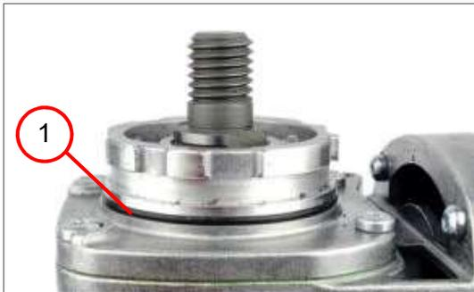
1. Remove the sealing ring (1).
