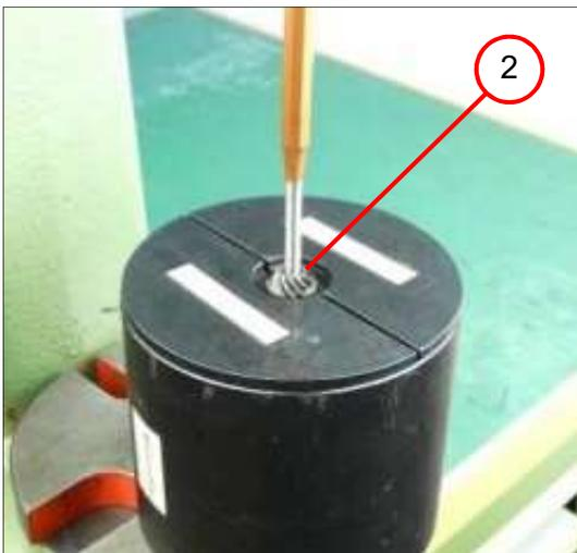
2. Remove the bevel pinion (2).
