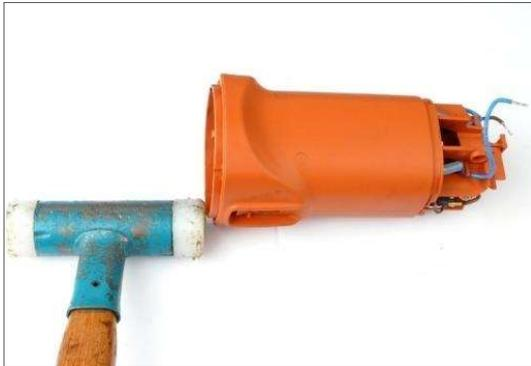
6. Remove the stator (1).
