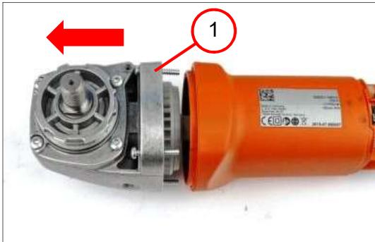
6. Remove the gearbox housing (1).
