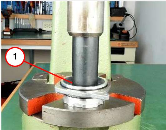
1. Press in the deep grooved ball bearing (1).
