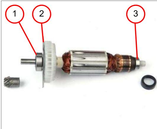
3. Remove the deep groove ball bearing (1).
