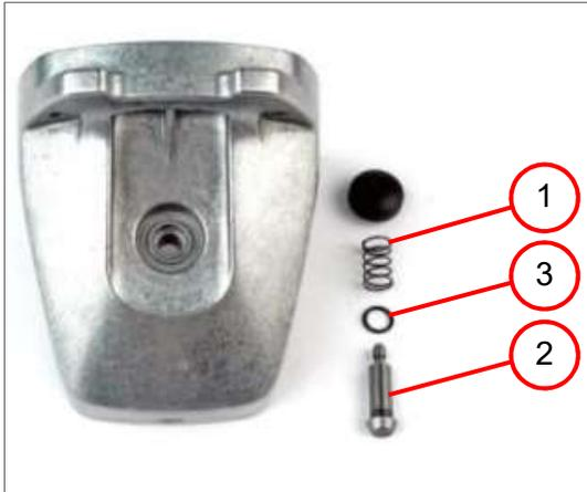
1. Insert the spiral spring (1) and the bolt (2) with sealing ring (3).
