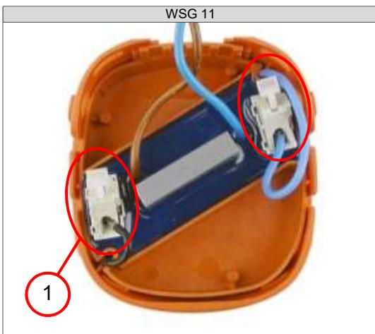
4. Open the two terminals (1) and connect the cables.
