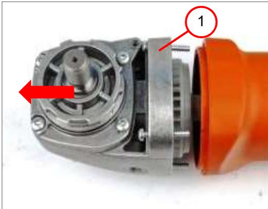
6. Remove the gearbox housing (1).
