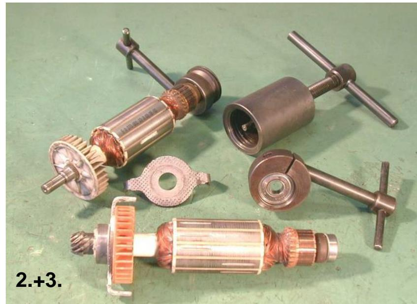
1. Lay armature pinion [\(170\)](#) in draw-off plate and press down using centre punch and a spindle press.
