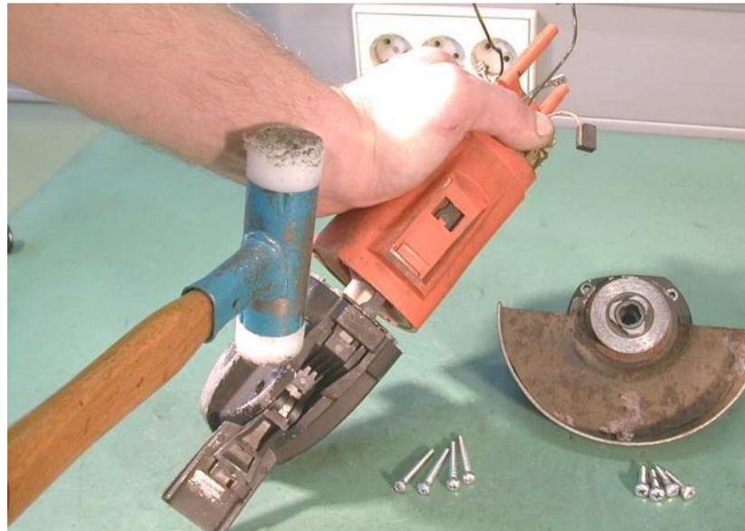
1. Screw out oval head screws [\(150\)](#) on the bearing plate [\(250\)](#).
