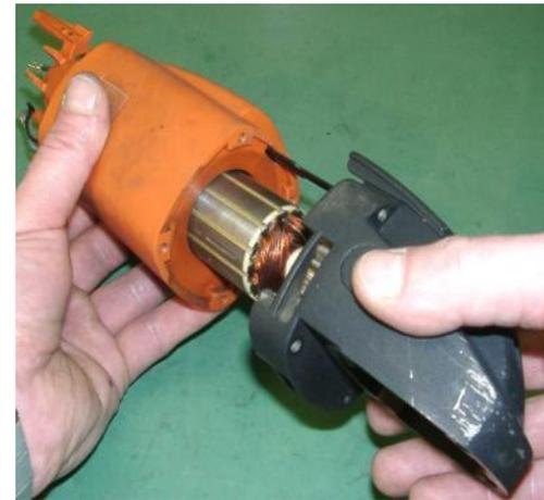
1. Set preassembled armature [\(100\)](#) into preassembled gear housing [\(430\)](#) by hand.
