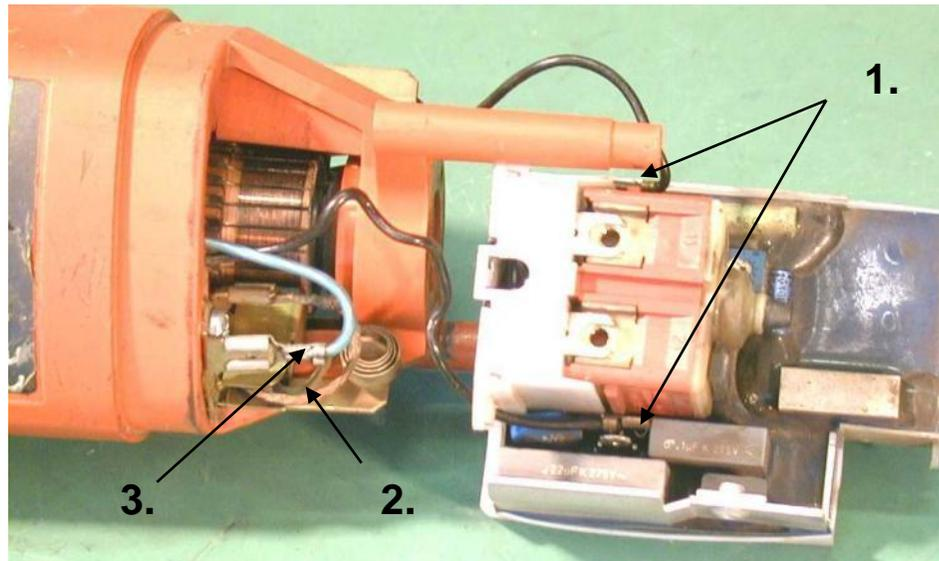
1. Pull field magnet cable from the electronics [\(40\)](#) and pull off electronics + pushed on circuit breaker [\(540\)](#).
