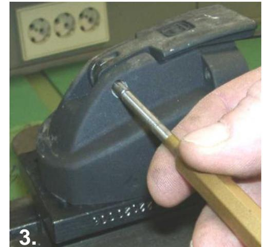
1. Place gear housing [\(430\)](#) in assembly fixture and plug in interlock [\(510\)](#) and holding spring [\(460\)](#).
