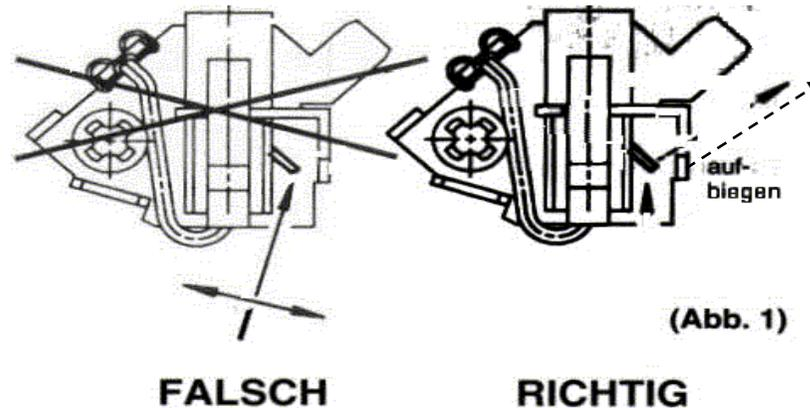
1. Mount carbon holder (60) supplied with carbon brushes (70) on motor housing (90) and connect.
