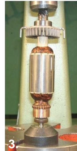
1. Place armature [\(100\)](#) into the pressing fixture with the collector side down. Put closure plate [\(120\)](#) on top and press on ball bearing [\(450\)](#) with the help of the ball bearing piece (D=26).
