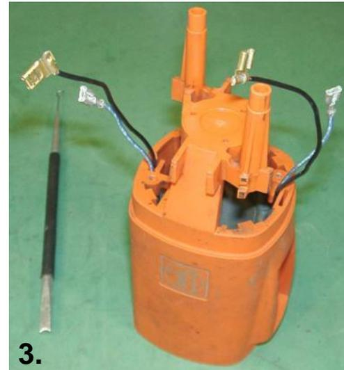
1. Place the 4 field magnet strands in the inside and insert field magnet [\(490\)](#) into the motor housing [\(90\)](#).
