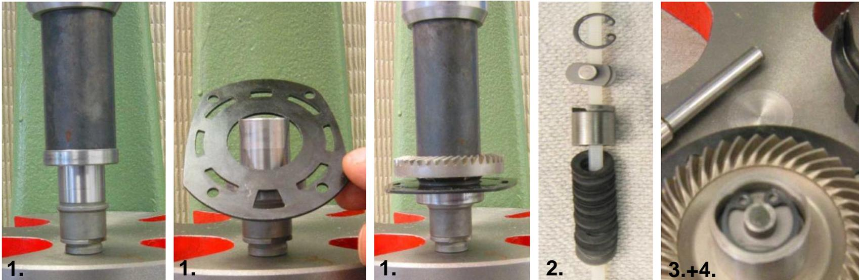
1. Press ball bearing [\(230\)](#) , closing plate [\(260\)](#) and bevel gear [\(280\)](#) onto shaft [\(300\)](#) using the sleeve (D=20.5).
