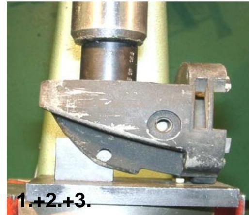
1. Lay gear housing [\(430\)](#) in pressing fixture.
