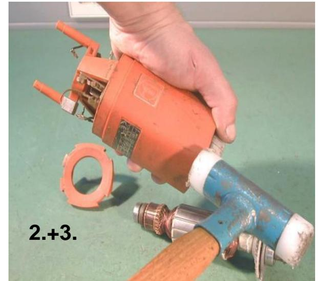
1. Loosen the gear housing [\(430\)](#) and the armature [\(100\)](#) from the bearing seat by hitting lightly against the motor housing [\(90\)](#), and/or against the gear housing [\(430\)](#).
