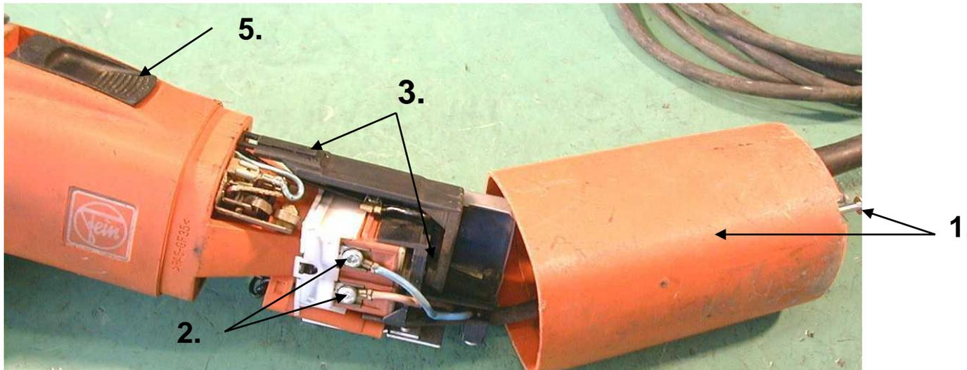
1. Loosen screws [\(500\)](#) and pull off housing cover [\(550\)](#).
