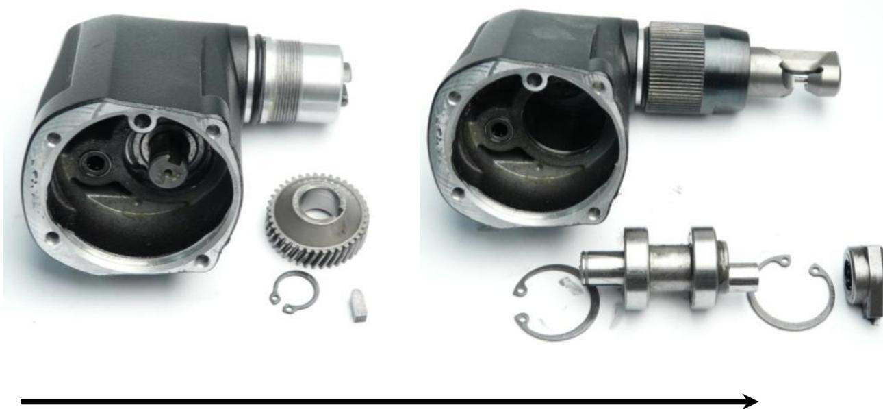
1. Remove circlip, gear-wheel and feather key.
