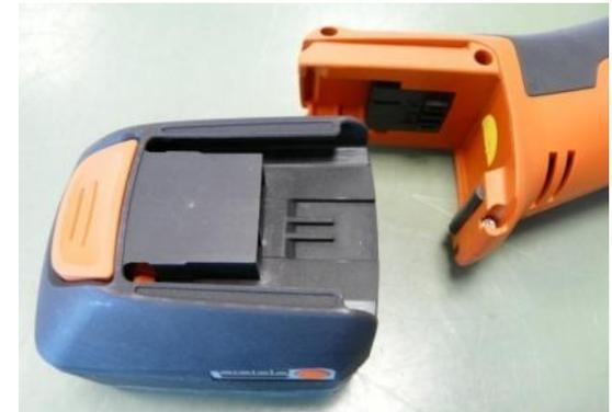
1. Press releasing button and pull out battery.
