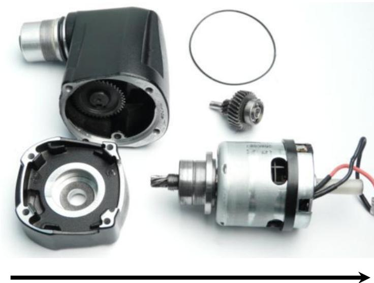
1. Pull intermediate bearing off gearbox head.
