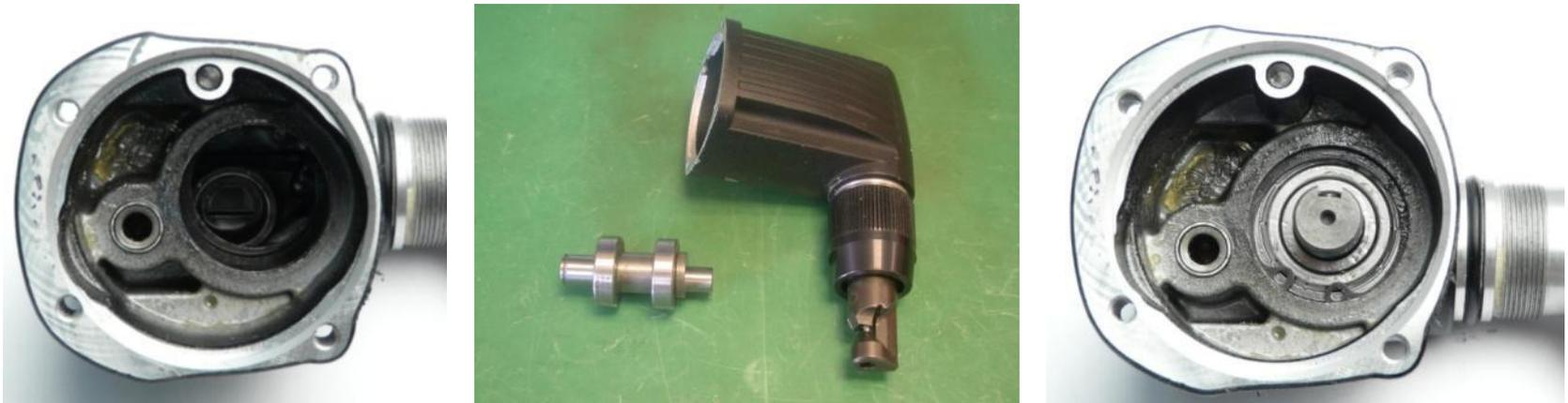
1. Fit drive together with needle sleeve in plunger.
