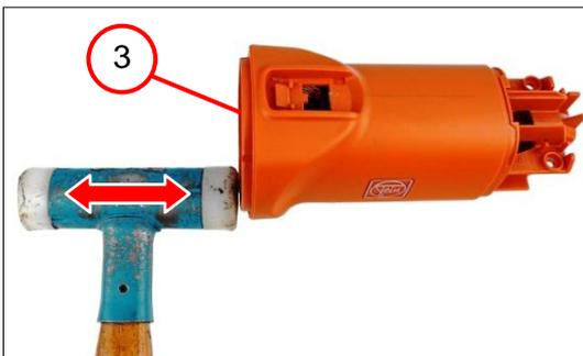
3. Remove the stator (3).
