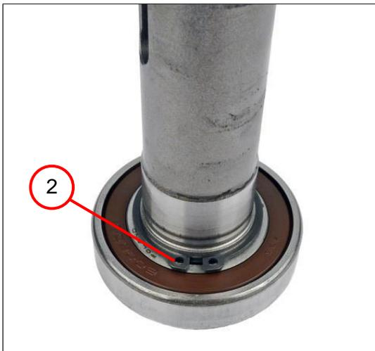
2. Position the circlip (2).
