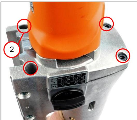
2. Screw in the four screws (2) [8.0 Nm  $\pm$ 0.3 Nm].
