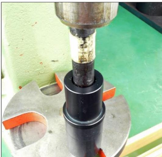
4. Press in the circlip (5).
