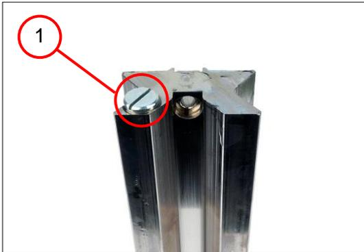
7. Screw in the flat-head screw (1) [1.2 Nm  $\pm$ 0.15 Nm].
