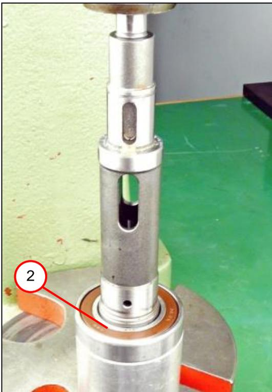
2. Press the deep groove ball bearing (2) off the shaft.
