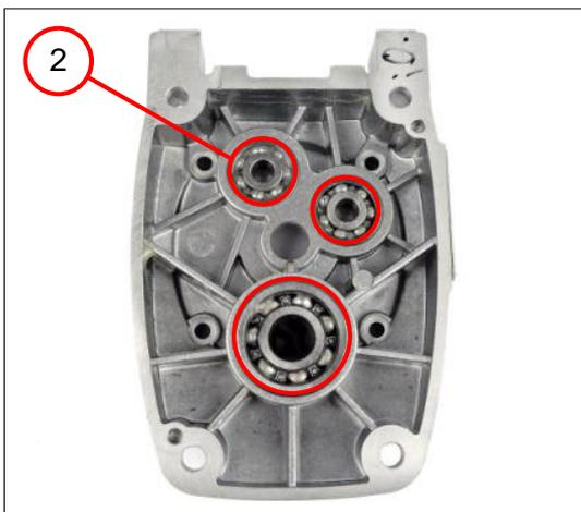
2. Remove the three deep groove ball bearings (2).
