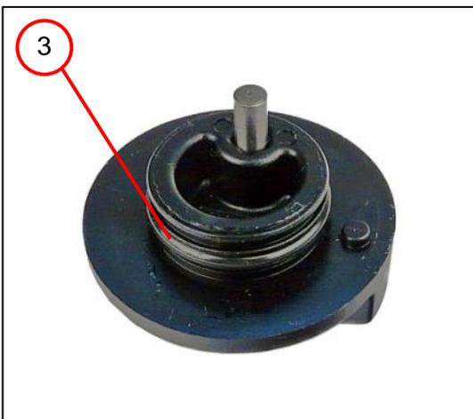
3. Remove the sealing ring (3).
