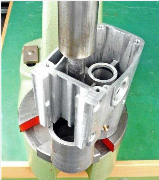
9. Press in the two deep groove ball bearings (1).
