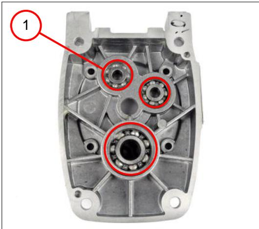
1. Press in the deep groove ball bearings (1).
