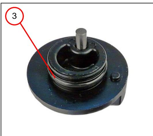
3. Coat the sealing ring (3) with oil.
