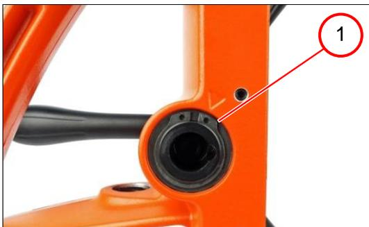
1. Remove the circlip (1).
