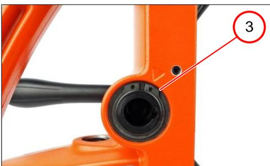
4. Position the circlip (3).
