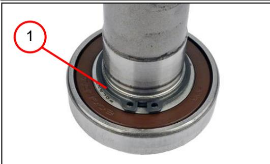
1. Remove the circlip (1).
