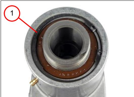
1. Remove the circlip (1).
