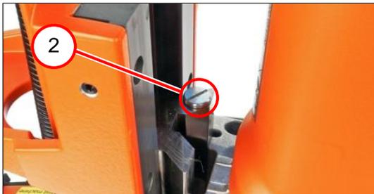
4. Screw in the flat-head screw (2) [1.2 Nm  $\pm$ 0.15 Nm].
