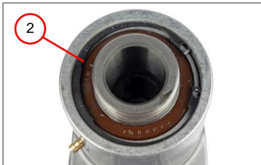
3. Position the circlip (2).
