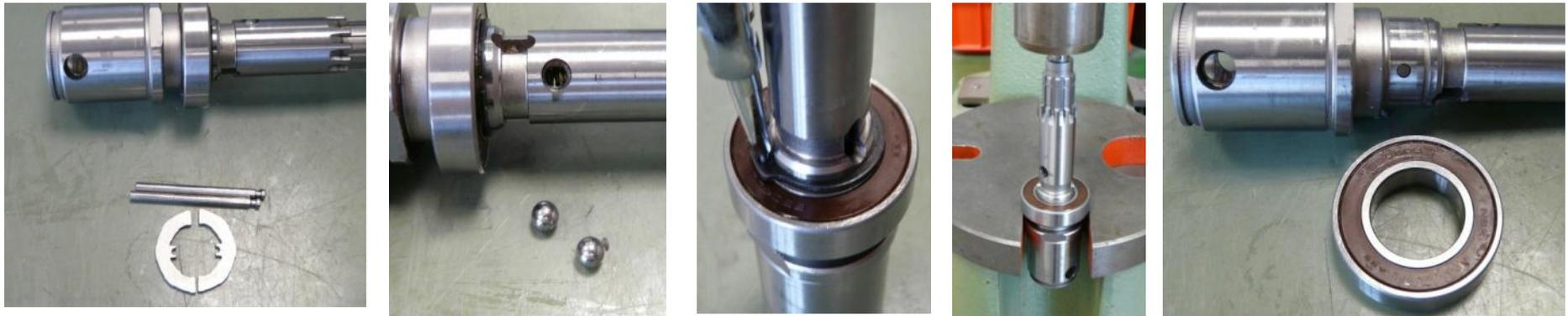
**Pull both bolts out of drill shaft from the front.
