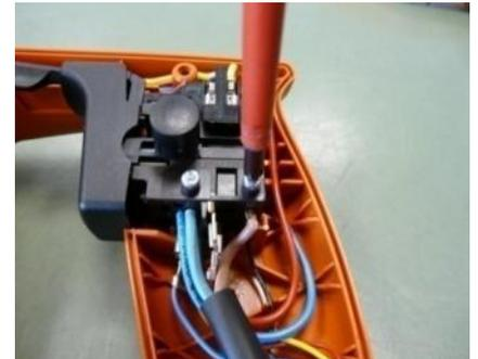
**Loosen screws and take off handle half shell.
