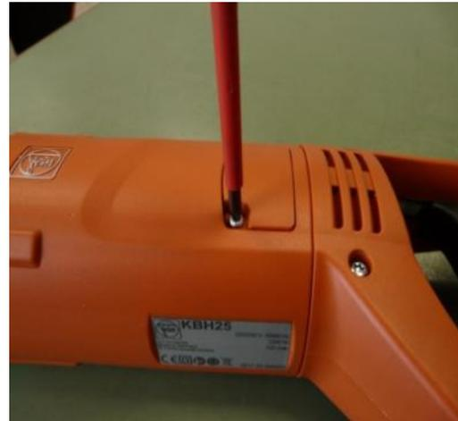
**Pull back spring and slide down carbon brush (attach on collector)**
