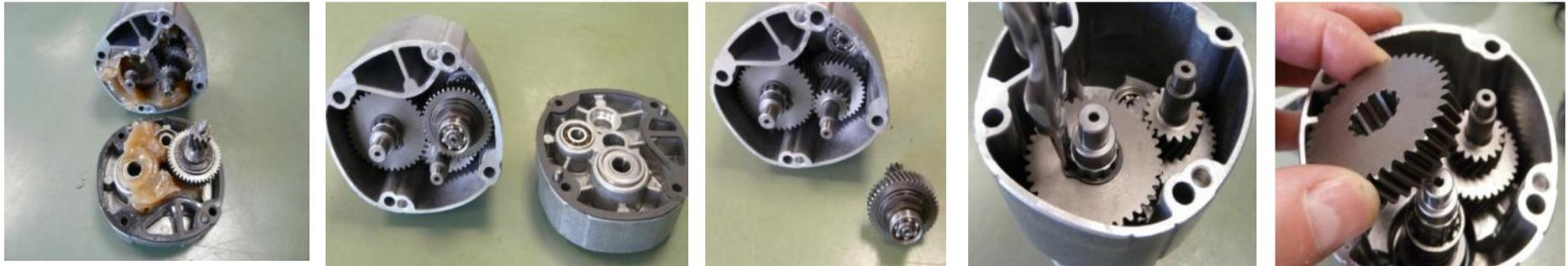
**Disconnect gearbox housing and intermediate bearing.
