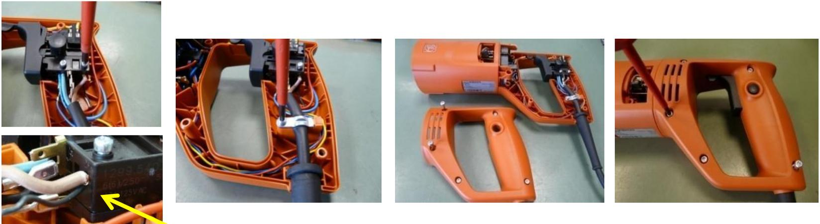
**Fit mains cable with stranded wire for restart protection (thin black cable)**
