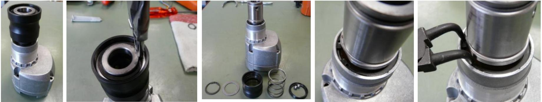
**Place gearbox housing on intermediate bearing.**
