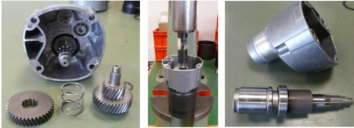
**Remove pressure spring and intermediate gear.
