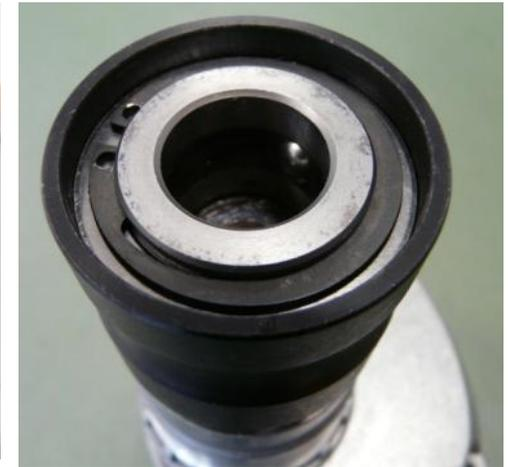
**Fix drill shaft in gearbox housing with circlip**
