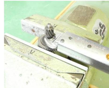
**Clamp slipping clutch in vice with aluminium jaws.**
