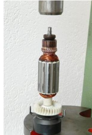
**Slide plate on to armature shaft**
