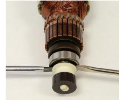
Drive armature out of intermediate bearing by tapping gently with a plastic hammer.
