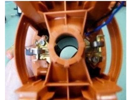
← Insert field coil up to stop in motor housing –
