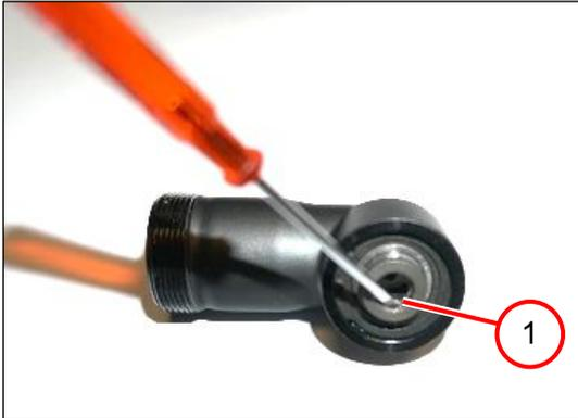
1. Position the circlip (1).
