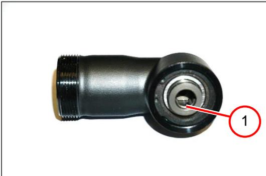
1. Remove the circlip (1).
